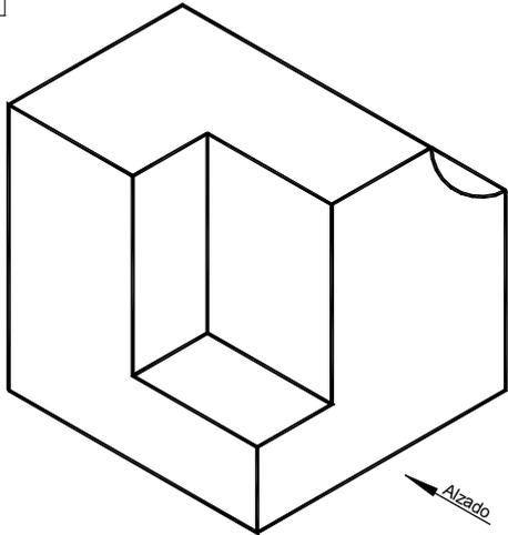
Isometric view of a rectangular block with a rectangular hole in the center. An arrow labeled "Alzado" points to the right, indicating the front view direction.
